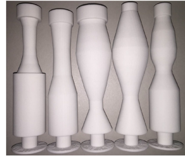
Figure 3: Replicated physical models of five Japanese vowels (from left: /i/, /e/, /a/, /o/, and /u/) [7].
